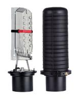
FOSC<sup>™</sup>450 D6 Fiber Optic Splice Closure, Gel Cable sealing, no pre-installed tray, 6 cable attach., three ground feedthrough lugs, with test valve
