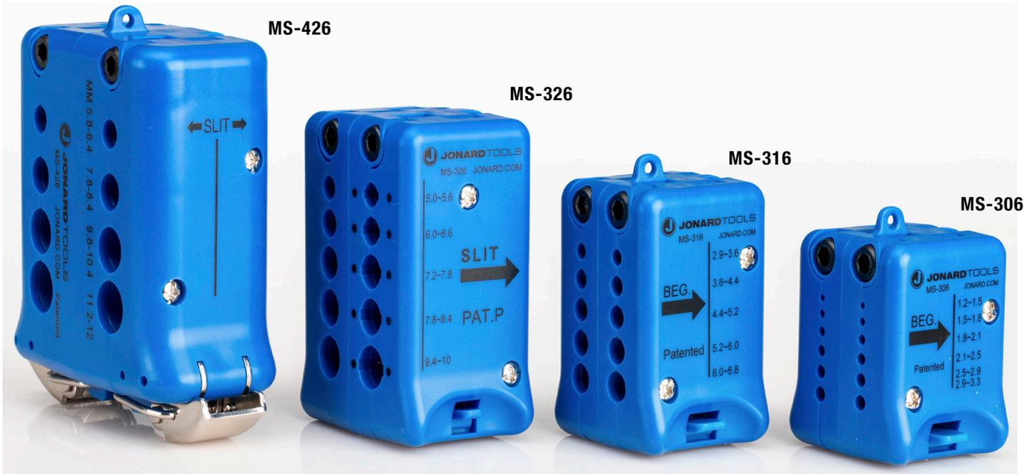
These **PATENTED** slit and ring tools are designed to open fiber jackets and loose buffer tubes to provide easy fiber access. One side of the tool slits fiber jackets and loose buffer tubes, the opposite side rings fiber jackets and loose buffer tubes. All this is done without damage to the fiber. Blades are replaceable. Note: MS-326 is designed for cables used in ducts and microducts.
